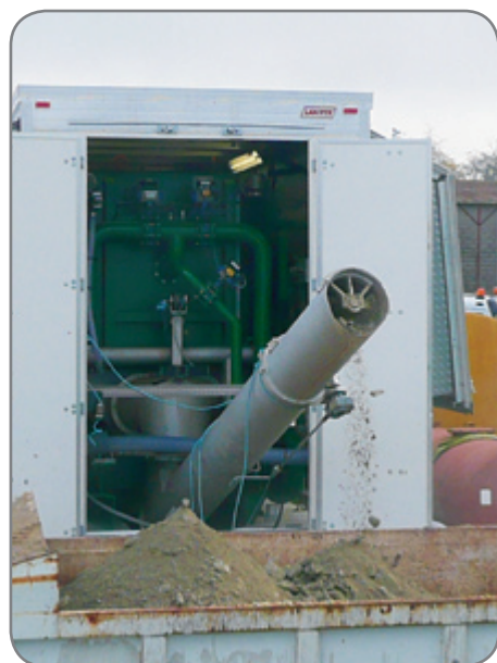
Cake removal by screw conveyor
